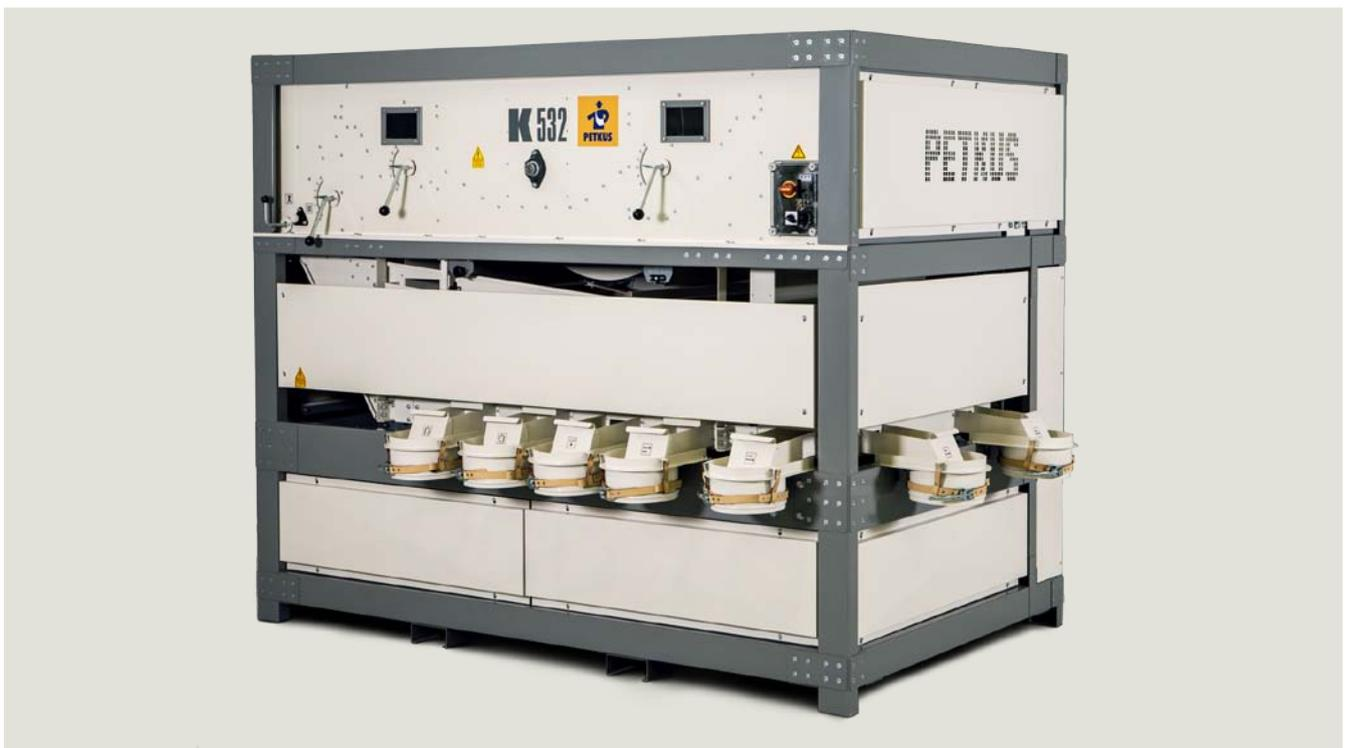
The **PETKUS seed cleaner K 532** is used for high-quality seed cleaning of free flowing bulky products, e.g. pulses which do not need to be processed with an indented cylinder. The high standard of cleaning is achieved by a combination of the screening process, the air aspiration system, and the indented cylinders.
