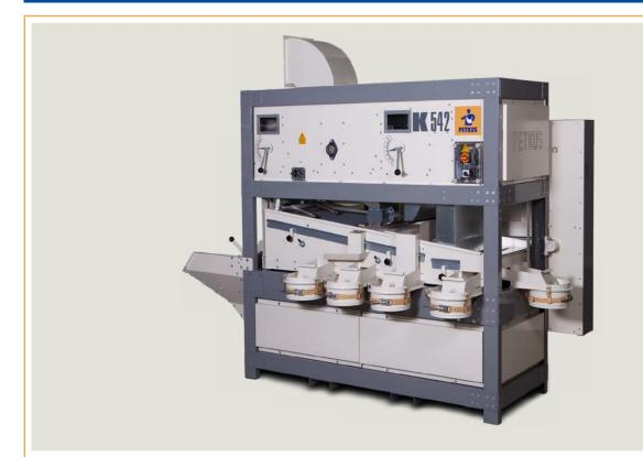
The **PETKUS Seed Cleaner K 542** is used for high-quality seed cleaning of free flowing bulky products, e.g. pulses which do not need to be processed with an indented cylinder. Furthermore, the seed cleaner can also be used for the intensive cleaning of grain, oilseeds, and pulses. The high standard of cleaning is achieved by a combination of the screening system and the air aspiration.
