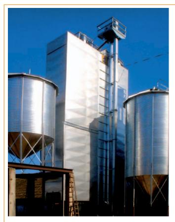
The **PETKUS Continuous Flow Dryers Type WS** are tower dryers designed for drying grain, oilseeds and seed. Four series (15, 25, and 40) are available.
